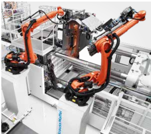
Two robots decouple heating of the organo sheet and demolding of the finished part – for short cycle times.
