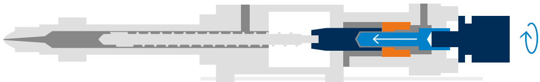
The proven in-line injection unit and innovative APC plus provide for extremely good shot weight consistency.
