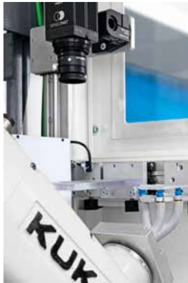
Quality control in a confined space – Integrated camera systems for component inspection.
