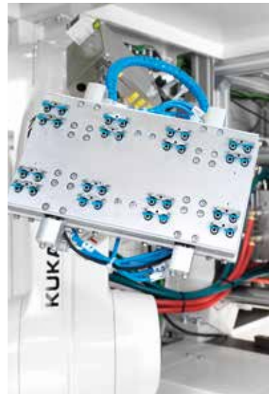
Our own gripper technology for the high-precision removal of 32 membranes with a wall thickness of only 0.2 millimeters.
