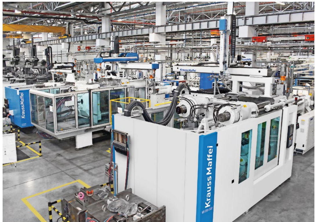
View of the machinery pool at Elba: In addition to the processing of BMC on the CX 420 Polyset, thermoplastic matrix materials are also processed on KraussMaffei machines. Photo: KraussMaffei
